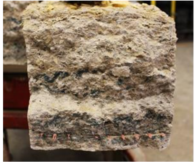
Figure 19. Flexural failure section textile-reinforced beam showing ruptured reinforcement and concrete layer inconsistency.
